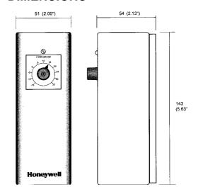
Dimensions in millimetres (inches in brackets)
